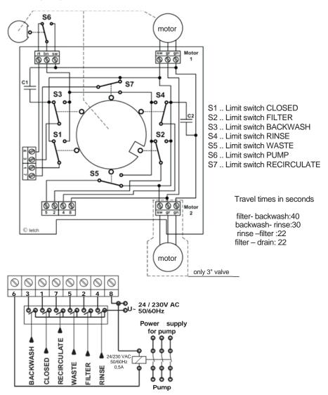
**Attention:** Only one position can be triggered, for example "FILTER" or "BACKWASH" but not "FILTER" and "BACKWASH" together!
