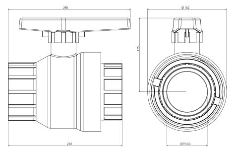
While other Ball Valves have a narrowed passage, the Netafim Ball Valve has a wide throat and clear pathway. This maximizes flow through when installed along a pipeline and increases flushing performance when installed on line ends.
