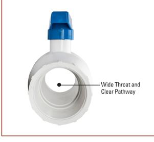
The solid one piece handle can be easily removed or replaced without tools. The 1" internal and 1 1/2" external hex shape of the stem allows the valve to be operated with a wrench or socket if the handle is removed.
